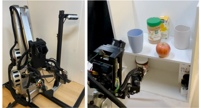
Fig. 1. Manipulation system setup. Left: Manipulation platform with 6-DoF arm, 6-DoF gripper, multimodal fingertip sensing, and Intel Realsense D435i camera. Right: Objects are picked from the upper shelf and placed in a dishes bin, on the lower shelf, or dropped into a trashcan.
