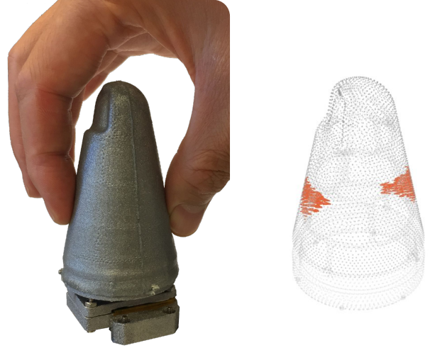
Fig. 1. We design a soft thumb-sized vision-based haptic sensor that gives detailed force distribution information over its 3D sensing surface.
